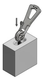
To transport the concrete units, the appropriate lifting system for the load group is inserted above the anchor head. Only matching components will fit together.
