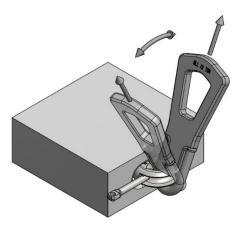
In this position, the connection element may lock inside the shackle. A small angle of the lifting cable angle will determine the bracket to bend. The problem can be overcome by turning the connection element. In this position, the connection element cannot lock.
