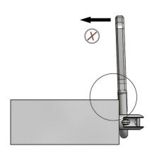
If the lifting direction is not heeded, the precast element or the lifting clutch can suffer major damage. Proper use can prevent damage and extend the service life of the lifting system.
