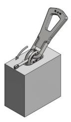
The lifting system is locked using a simple handle on the locker. The lifting system is now free to move in any direction. From this moment, the precast concrete unit can be lifted out of the formwork and transported to the storage site.
