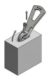
After the lifting/transport of the precast element, the lifting system can be easily released by pushing back the locker after the system is off load. The lifting clutch can remain attached to the crane hook until further use.
