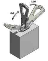
Angled pull using cable or chain with  $\beta > 45^{\circ}$  is not allowed.
