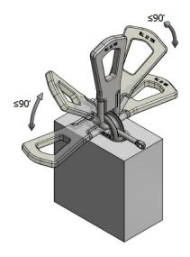
The clutch's 2D lifting bracket can be moved in any direction. Overloading the lifting anchor is not permitted (see the 2D lifting anchors conditions).
