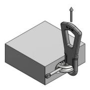
The flat precast concrete units can be moved from the horizontal to vertical position by using TILT UP anchor SA -TU or SA -TTU with additional reinforcement embedded in concrete. The direction of pull is at right angles to the cast-in anchor. Using a crossbeam for lifting to avoid angular and torsion forces is recommended.
